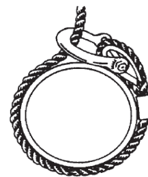
Correct – Shackle pin cannot turn.
