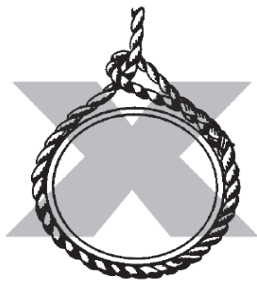
Incorrect – Cutting action of eye splice on running line.
