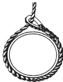
Correct – Use thimbles in the eyes.
