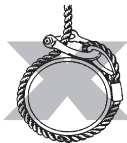
Incorrect – Shackle pin bearing on running line can work loose.
