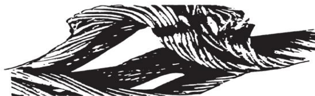
A birdcage which has been forced through a tight sheave.
