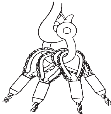
Whenever 2 or more ropes are to be Placed Over a Hook – Use a Shackle
