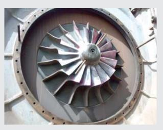
A new impeller was installed in the first stage process gas compressor
