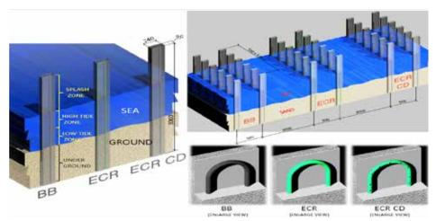
BB- Black Bar, ECR- Epoxy Coated Rebar, CD – Controlled Damage FIGURE-3
