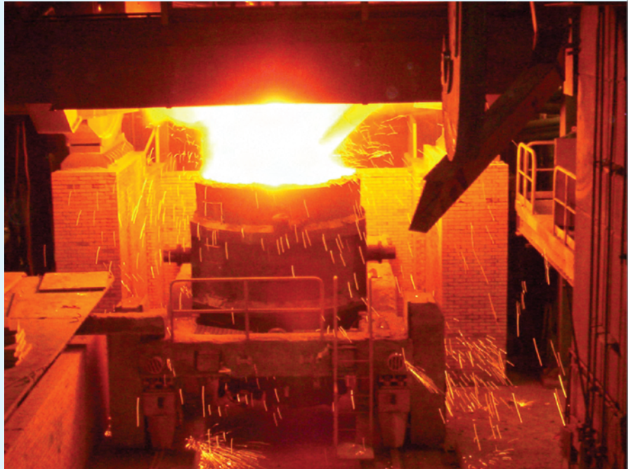
View of the Electric Arc Furnace: First heat is being tapped
